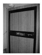
The refrigerator operates on 120-volt AC power or propane. The operating instructions supplied in the Owner's Information Package will help you with detailed information from the manufacturer.
