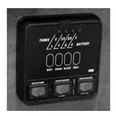
The systems monitor panel incorporates controls for the water and holding tank levels, battery condition and water pump. It may also control the water heater.
