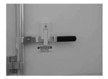
To open the bed door, depress the latch and pull the bar lock lever down on one of the latches. Move to the other side and while supporting the door, repeat the process. Carefully lower the door until it has extended into the bed position.
