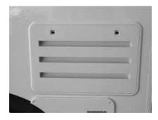
The Refrigerator Vent/Door provides access to the rear of the refrigerator for service and supplies inlet ventilation for proper operation.
