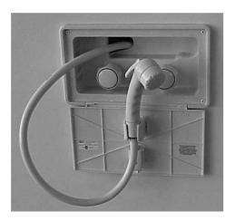
The exterior wash station is located in the service center on the roadside compartment for exterior use. It uses water from the fresh water tank or when connected to the city water hookup. The showerhead is equipped with a flow control to allow you to conserve water. This flow control is not a permanent shut off.
