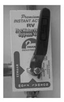
The water heater bypass valve is located behind the water heater and is used when winterizing the water system for storage. By rotating the lever to the bypass position, antifreeze will not enter the water heater requiring less antifreeze to protect the water system plumbing. Follow the instructions shown on the valve.
