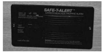
Refer to the section on Fire and Safety, on the operation of the Combo Carbon Monoxide & Propane Leak Detector.
