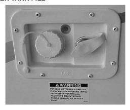
The fresh water system should be sanitized at the initial filling, after a period of storage or if contaminated. See "Sanitize Fresh Water System" in this section. Fill tank slowly. Do not overfill. Do not leave unattended while filling. Structure damage may occur.
