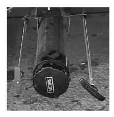
The holding tanks terminate in a valve arrangement that permits each tank to be dumped separately or together. The valves are called "knife valves". A blade closes the opening in the sewer drain pipes. The blade is connected to an extension handle that is pulled to release the contents of the tank(s).
