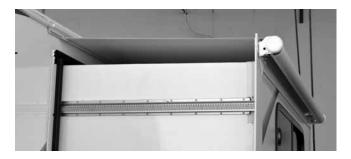
The slideout cover extends and retracts with the slide room. It helps to divert water off the slide room roof and helps in keeping the roof clean of debris. The room seal can become less effective or even damaged if the slide room roof is not kept clean.
