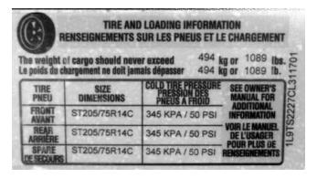
The first (upper) label is the Tire and Loading Information Tag. It lists the trailer VIN number and maximum cargo capacity of the trailer as equipped by Lance. It also lists the tire size and Cold Tire Pressure of the tires that are supplied on your trailer.
