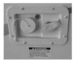
The city water inlet connection is located on the roadside of your trailer.
