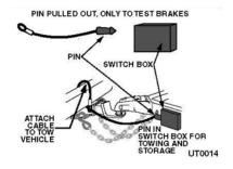
If the coupler or hitch fails, a properly connected and working breakaway switch will apply electric brakes on the trailer. The safety chains will keep the tow vehicle attached and as the brakes are applied at the trailer's axles, the trailer/tow vehicle combination will come to a controlled stop.
