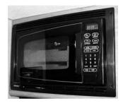
Please read all instructions that come with the convection or microwave oven before use. The oven should never be operated empty. When operating on your generator (if equipped) power is limited. If the roof air conditioner is operating there may not be enough power to operate the microwave.
