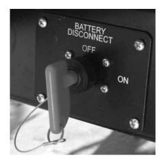
Your trailer is equipped with a battery disconnect switch. Switching the lever to the "OFF" position will disconnect/isolate the battery from the rest of the 12V electrical system.
