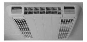
The roof-mounted Air Conditioner operates on 120-volt power, which is supplied through the 30-amp power cord, either from an outside 120-volt power service or by the onboard generator, if equipped.
