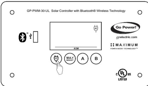
Now you can turn the connected inverter on or off by holding down the **AC Symbol Button** for 3 seconds.
