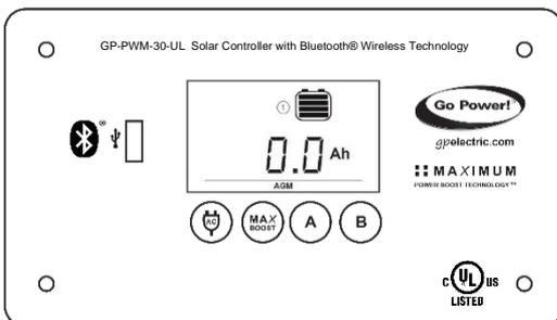
To reset the count of ampere hours charged, use the Go Power! Connect app (Bluetooth® enabled version only).
