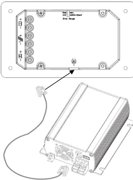
First, connect the inverter directly to the battery (follow the installation instructions included with the inverter). Then, connect the modular cable (found in the inverter remote box) to the remote terminal of the inverter and to the remote terminal of the GP-PWM-30-UL (marked with an **AC Plug symbol**).
