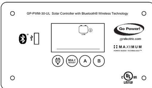
**Low battery 2:** If there are two battery banks connected and the SOC of battery bank 2 reaches 0%, the battery SOC symbol will show the text “LOW” beneath it. The controller will continue operating in this condition and will only stop operating if the voltage of Battery 1 drops below 9.0 VDC (this is because the GP-PWM-30-UL is powered by Battery 1).
