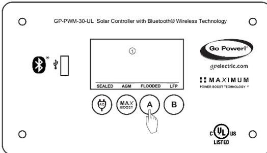
Next, select the charging profile of battery bank 1 by pressing the **B Button** to toggle through the profile options: Sealed/Gel, AGM, Flooded, or LFP.
