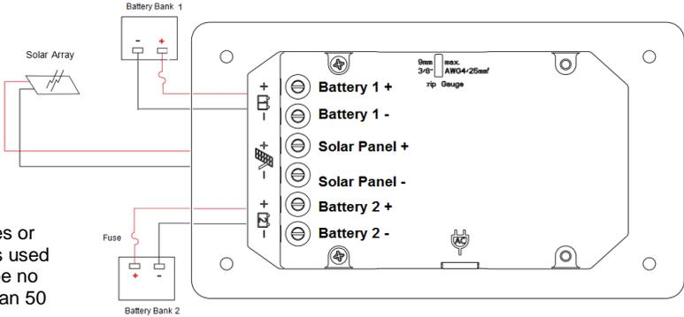
The fuses or breakers used should be no larger than 50 amps.
