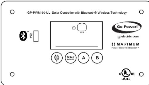
**Low battery 1:** If the SOC of battery bank 1 reaches 0%, the battery SOC symbol will show the text “LOW” beneath it. The controller will continue operating in this condition and will only stop operating if the voltage of Battery 1 drops below 9.0 VDC.
