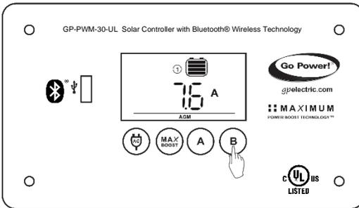
Push the **B Button** to show the PV charging current for battery 1. The GP-PWM-30-UL will begin to limit the current as Battery 1 reaches a full charge. The current that is not used for Battery 1, is used to charge Battery 2.
