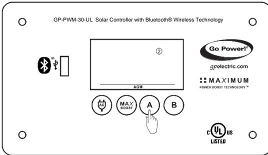
To select the charging profile of battery bank 2, press the **B Button** to toggle through the profile options: Sealed/Gel, AGM, Flooded, or LFP.
