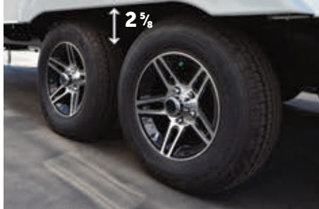
Available Chassis Lift Kit Provides an Additional 2 5/8" of Clearance
