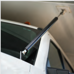
Exclusive Lance cabover struts cut down on sway from wind. - Remove during off-road use
